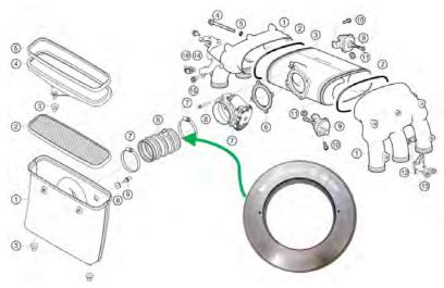
991-2 Cup cars must be fitted with a 55 mm diameter air flow restrictor reference MR001442 installed on the intake according to the diagram below.
